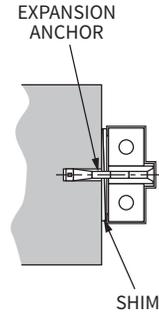
Figure 21: Existing Masonry or Poured Concrete Wall Anchorage
