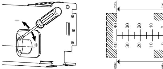
Figure 23: Adjust Spring Tension.
