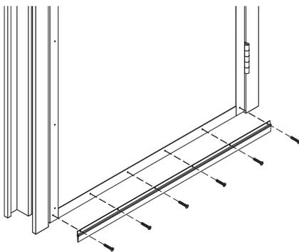
Figure 23: Sweep Gasket Installation
