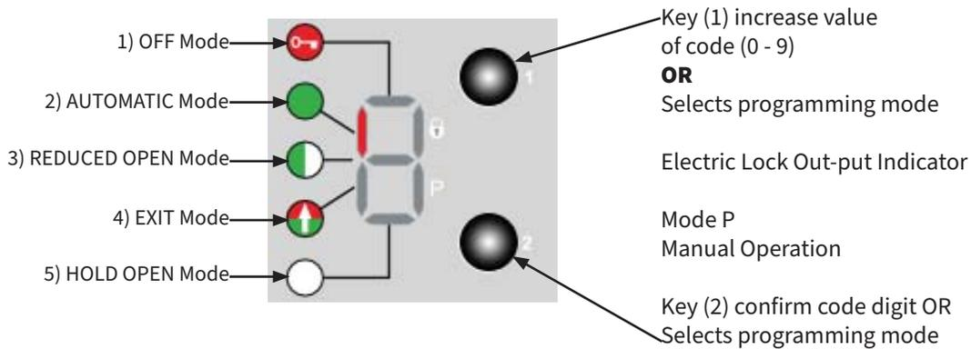
Figure 08: Operation of FCP Control Panel
