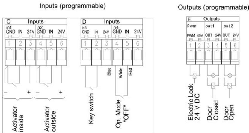
Figure 18: Single Swing Inputs & Outputs
