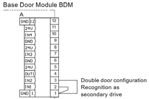
Figure 16: Secondary Drive Wiring.
