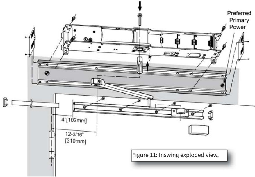
Figure 11: Inswing exploded view.
