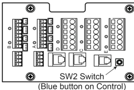
Figure 13: "SW2" switch on Control
