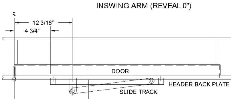
Figure 05: Inswing Operator, W/SS Arm
