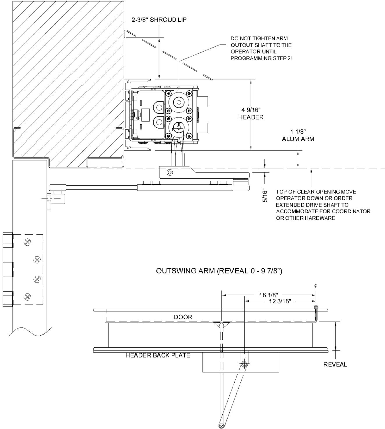
Figure 02: Outswing Operator, W/Aluminum Arm
