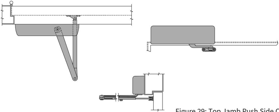
Figure 29: Top Jamb Push Side Closer
