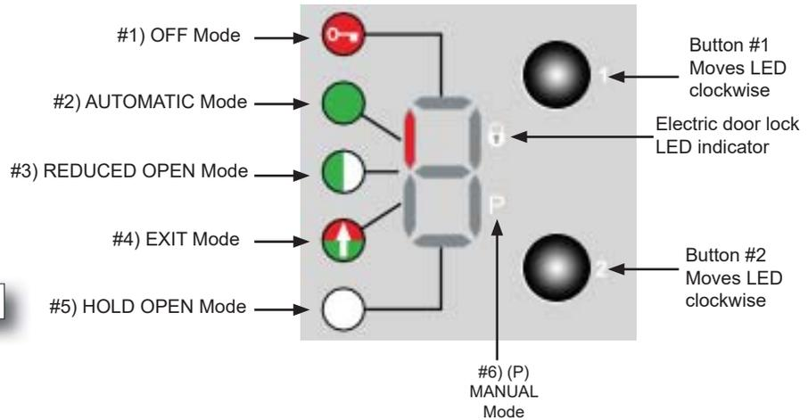
Figure 2: 6-Position Functional Control Panel.
