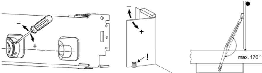
Figure 22: Adjust Internal Stop.
