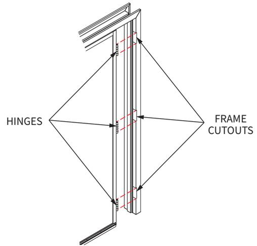
Figure 22: Panel Installation
