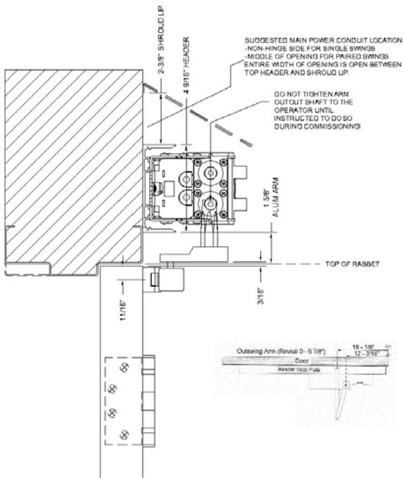
Figure 12: Standard Aluminum Inswing Arm.
