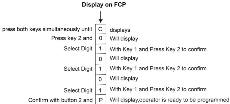
Example 2: Enter access code 103 to adjust the hold open time for 2 seconds
