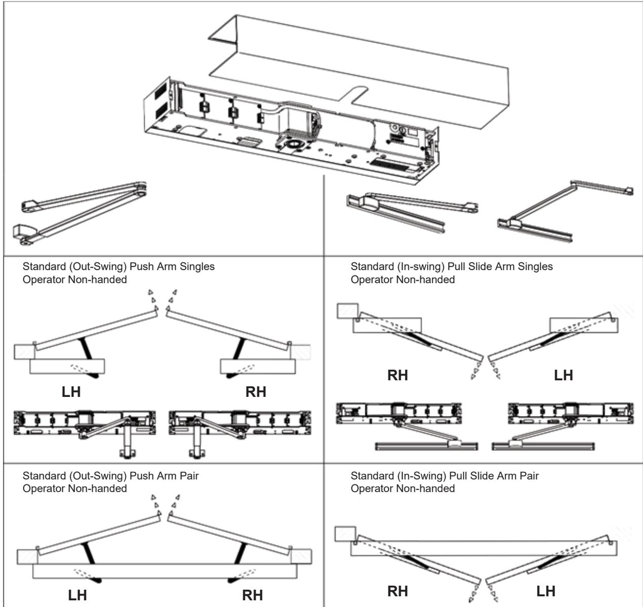
Figure 3: Door Operator Layouts.
