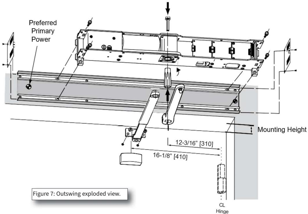
Figure 7: Outswing exploded view.
