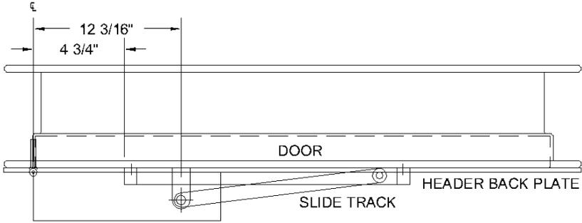
Figure 03: Inswing Operator, W/Aluminum Arm
