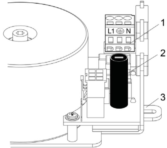
Figure 06: Main Power Connection
