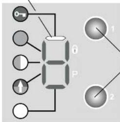
Press Button 1 and 2 simultaneously until "C" appears
