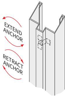
Figure 8: Drywall Tension Anchor
