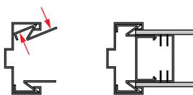
Figure 9: Snap-In Anchor
