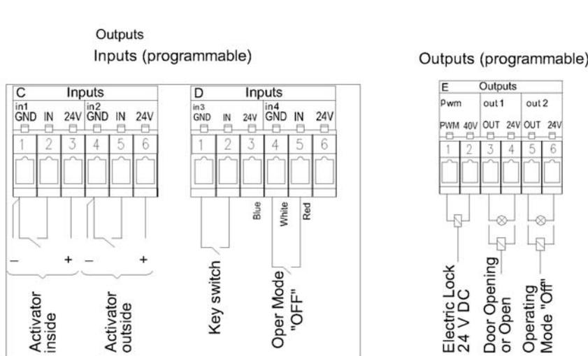
Figure 19: Paired Swing Primary Leaf Inputs & Outputs
