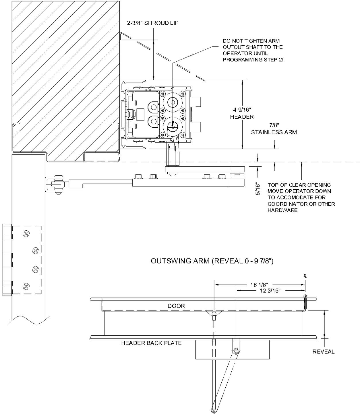
Figure 04: Outswing Operator, W/SS Arm
