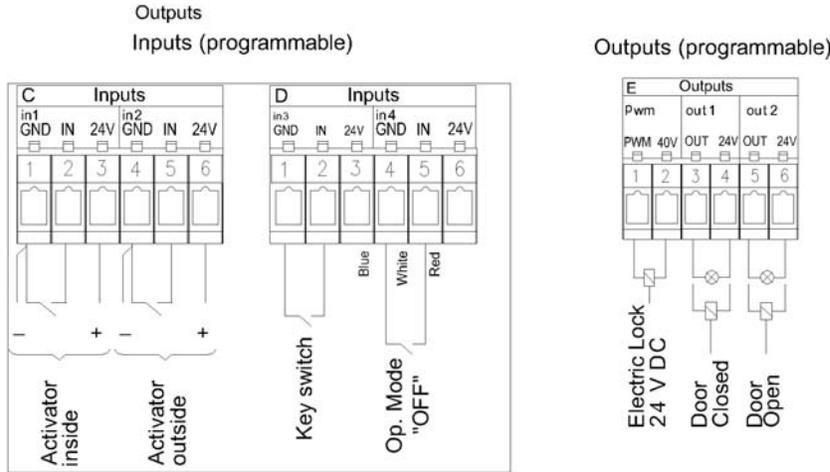
Figure 20: Paired Swing Secondary Leaf Inputs & Outputs
