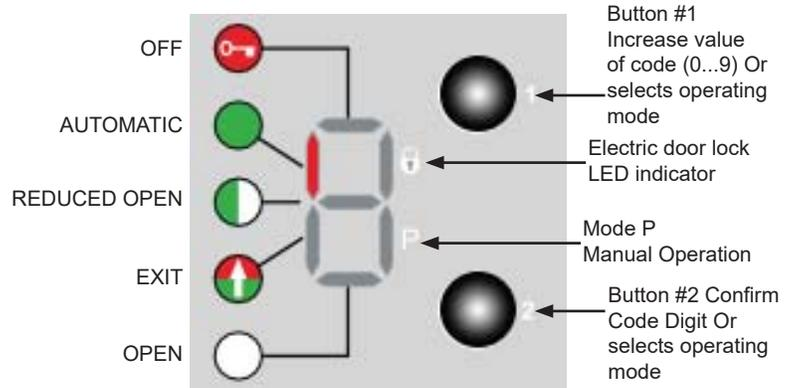
Figure 25: 6-Position Functional Control Panel.
