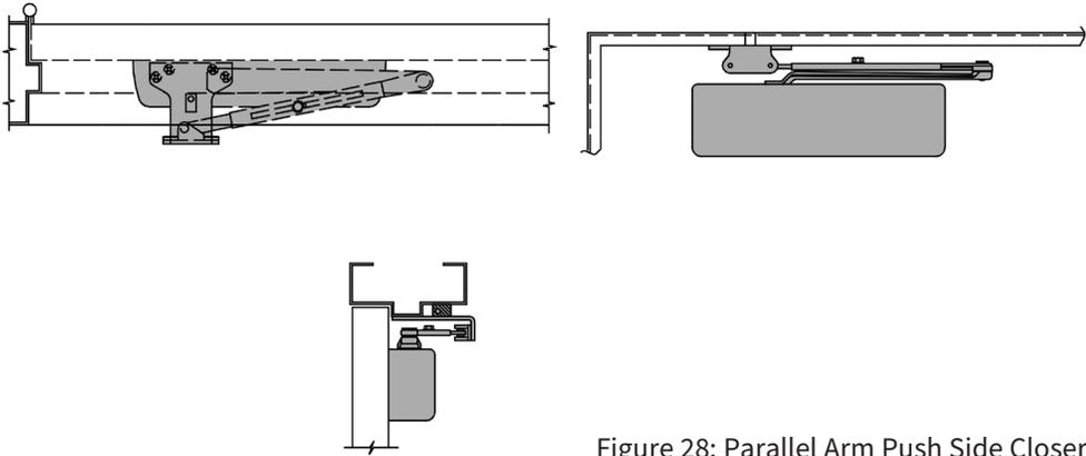
Figure 28: Parallel Arm Push Side Closer
