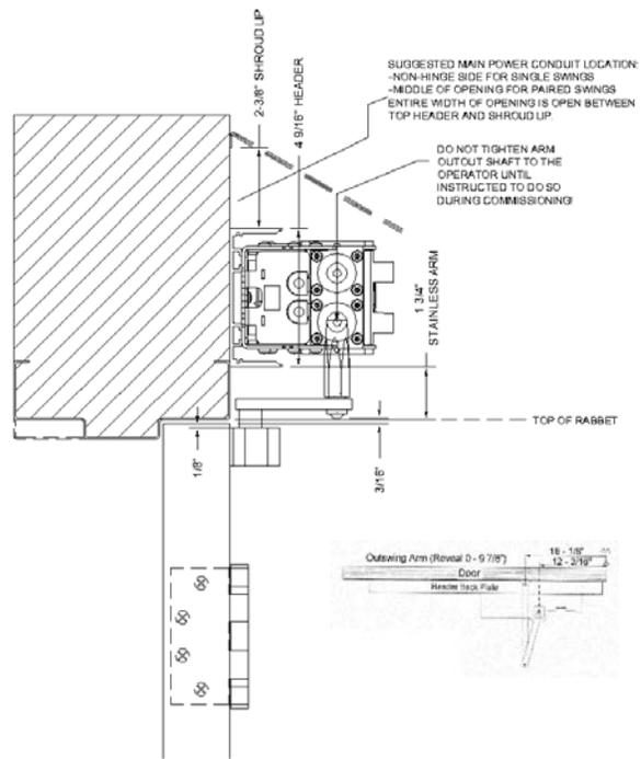
Figure 13: Stainless Steel Inswing arm.
