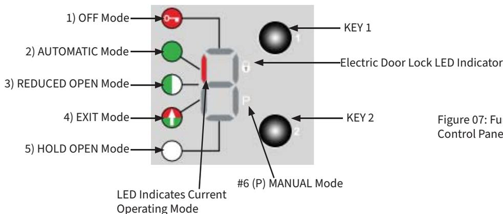
Figure 07: Functional Control Panel (FCP)
