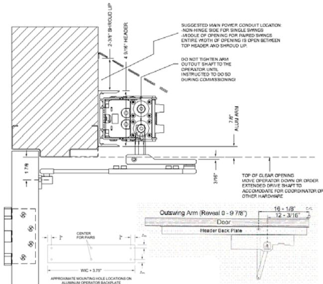
Figure 8: Standard Aluminum Outswing Arm.
