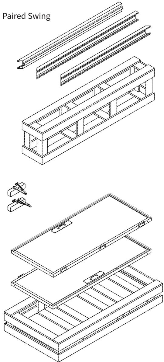
Upon receipt of the shipment, check that you have received the correct number of pieces as shown in (Figure 1). Crate one will contain the door panel(s). Crate two will contain the frame, operator and loose parts. **For your protection, note any damages or shortages on the carrier's bill of lading before signing the bill for receipt.**
