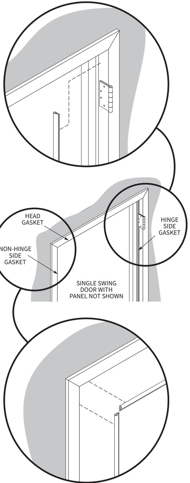
Figure 25: Frame Gasket Installation
