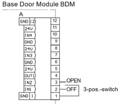
Figure 15: Primary Drive Wiring.
