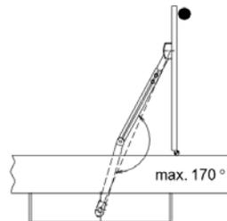
Figure 28: Adjust Internal Stop.
