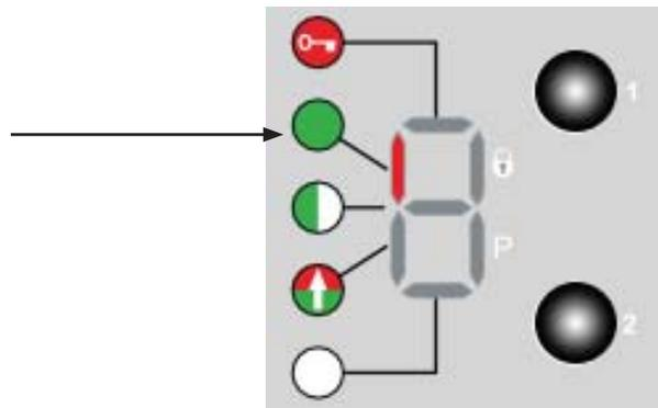
Figure 17: FCP "Automatic" mode (both Operators)
