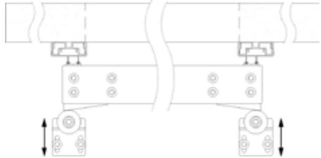
Figure 26: Adjust Floor Roller Position
