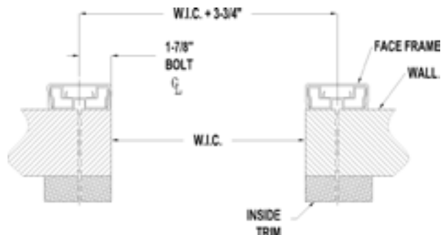
Figure 4: Wall Clip Position - Frames with Inside Trim
