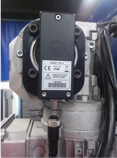
Figure 35A: Attach Encoder Cable
