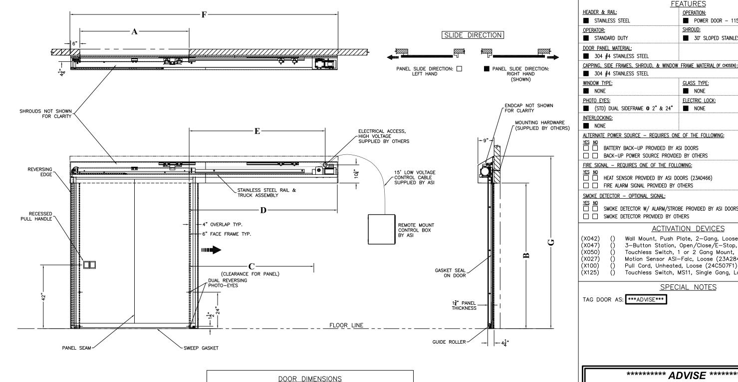
IF USING A JUNCTION BOX TO BRING POWER TO THE OPERATOR USING THE SUPPLIED HEADER CUTOUT, BOX MUST BE FLUSH WITH THE WALL AND WIRING MUST NOT INTERFERE WITH THE DOOR MOTION.
