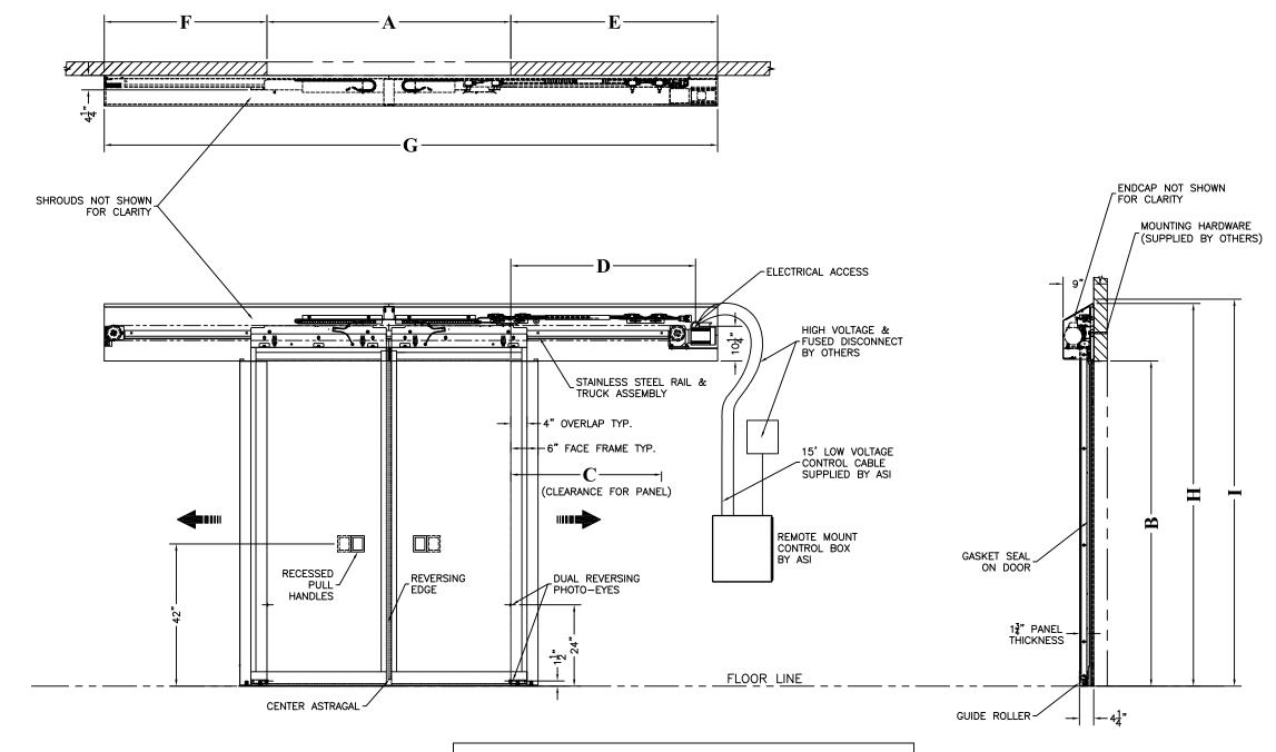
DOOR DIMENSIONS FINISHED OPENING WIDTH 6'-0" FINISHED OPENING HEIGHT В 8'-0" 3'-10 1/2 A/2 + 10 1/2" С A/2 + 18 1/2D 4'-6 1/2' A/2 + 255'-1" A/2 + 124'-0" 2A + 37'G 15'-1Н 9'-5" B + 17"B + 18 1/49'-6 1/4
